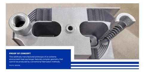
It's called additive manufacturing because you build a part and a material, one layer at a time. You're adding material, microlayer by microlayer, as opposed to subtractive manufacturing, which [includes many] traditional processes.
