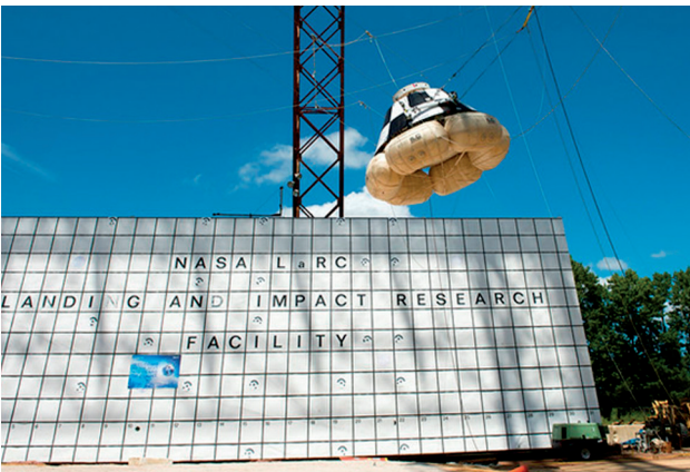
Land Landing Qualification Test campaign at NASA's Langley Research Center.
