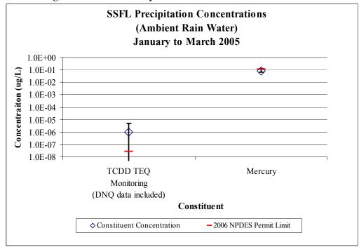
Figure 3 – SSFL Precipitation Constituent Concentrations
