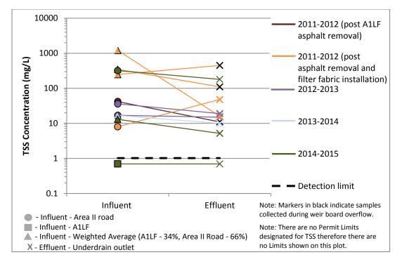
Figure 5. TSS at CM-9, post improvements (removal of A1LF asphalt and addition of CM weir board filter fabric)
