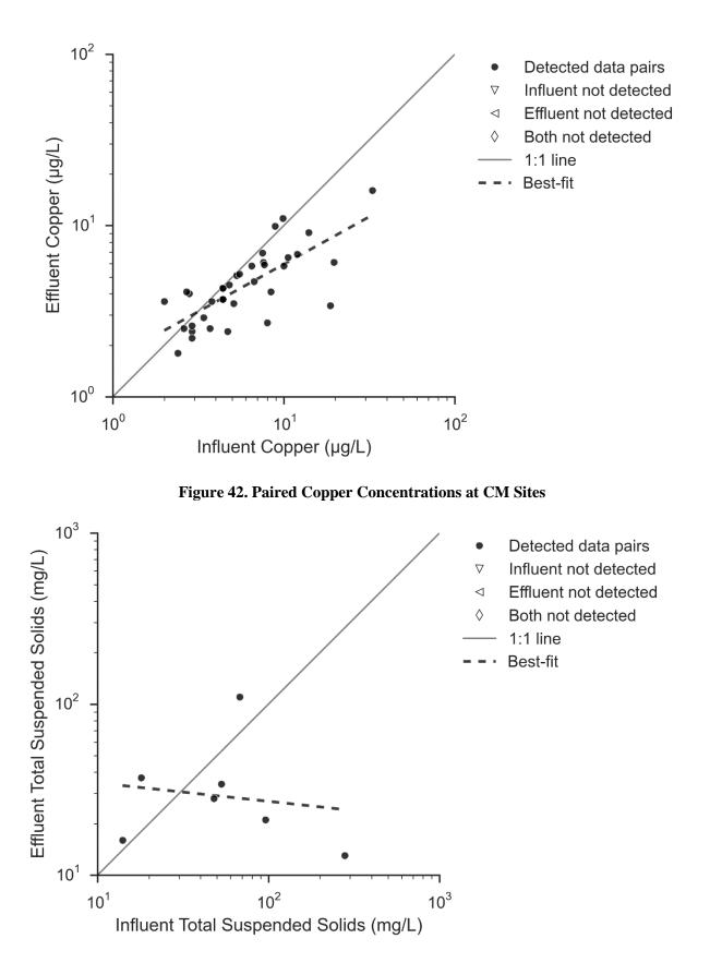
Figure 43. Paired TSS Concentrations at Lower Lot Biofilter
