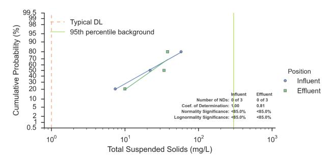
Figure 59. Probability Plot of TSS at ELV Stormwater Treatment BMP
