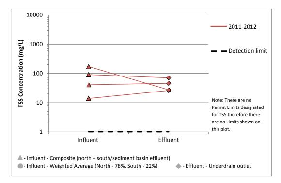
Figure 7. TSS at B-1 Media Filter (CM), pre curb cuts
