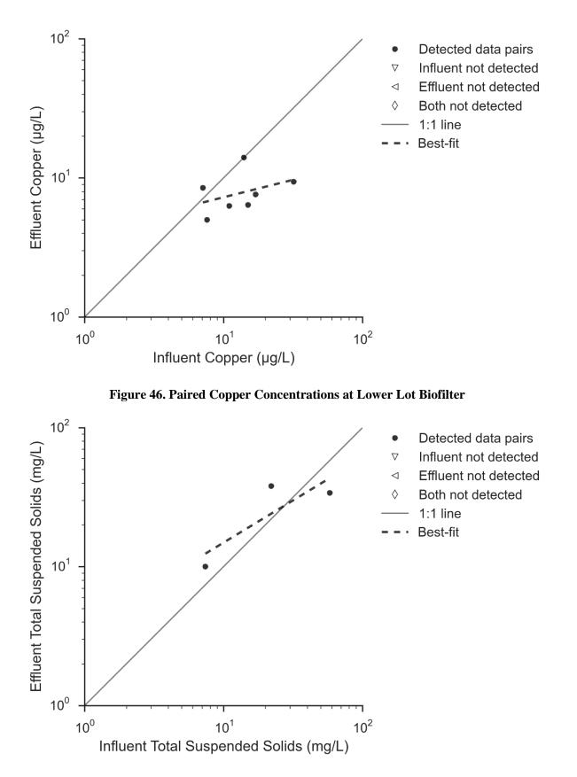
Figure 47. Paired TSS Concentrations at ELV Stormwater Treatment BMP
