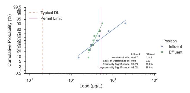
Figure 57. Probability Plot of Lead at Lower Lot Biofilter
