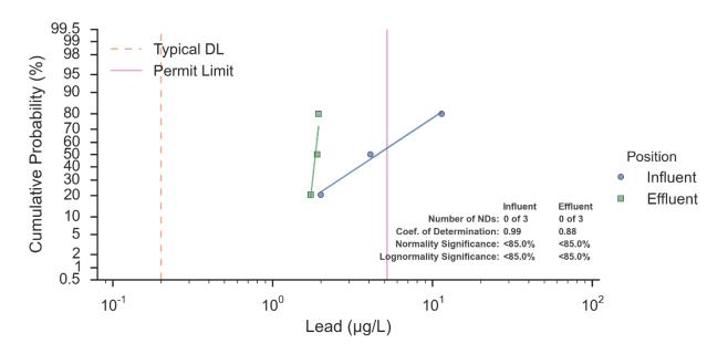
Figure 61. Probability Plot of Lead at ELV Stormwater Treatment BMP
