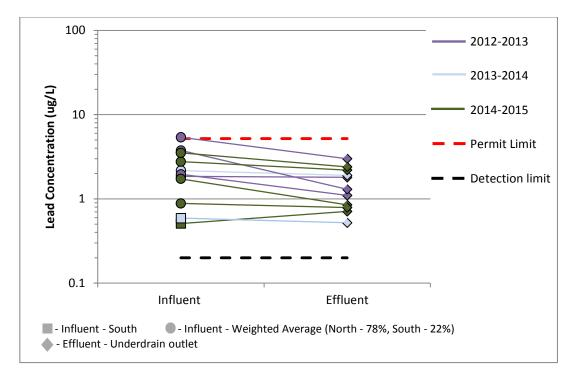
Figure 27. Lead at B-1 Media Filter (CM), post curb cuts
