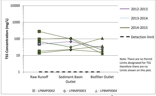
Figure 10. TSS at Lower Lot Biofilter<sup>7</sup>
