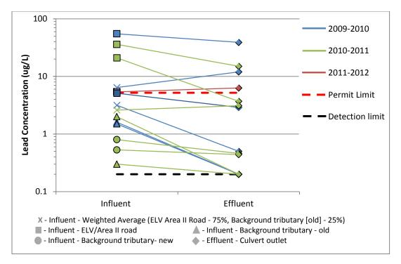
Figure 21. Lead at CM-1, pre filter fabric installation
