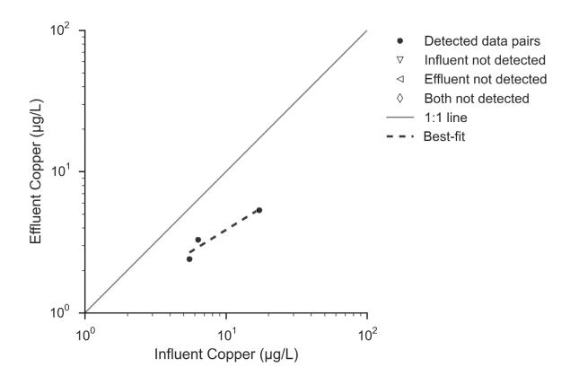
Figure 50. Paired Copper Concentrations at ELV Stormwater Treatment BMP
