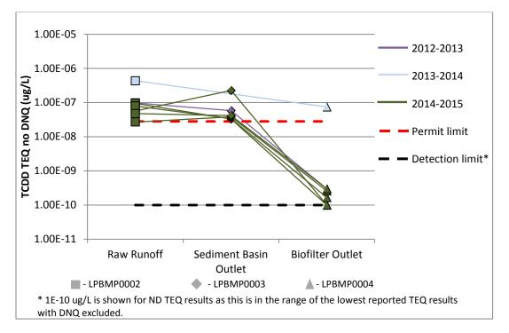
Figure 20. Dioxins at Lower Lot Biofilter<sup>7</sup>
