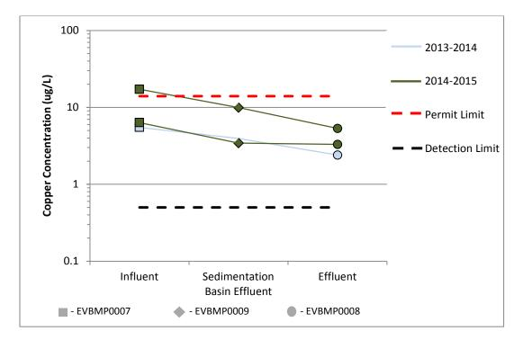
Figure 36. Copper at ELV Treatment BMP
