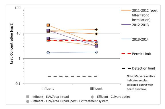
Figure 22. Lead at CM-1, post filter fabric installation
