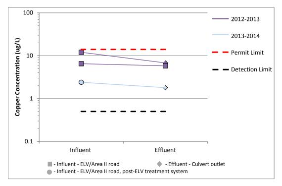
Figure 31. Copper at CM-1, post filter fabric installation
