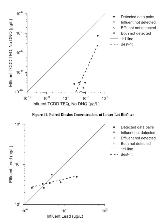
Figure 45. Paired Lead Concentrations at Lower Lot Biofilter
