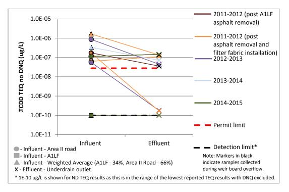
Figure 15. Dioxins at CM-9, post improvements (removal of A1LF asphalt and addition of CM weir board filter fabric)
