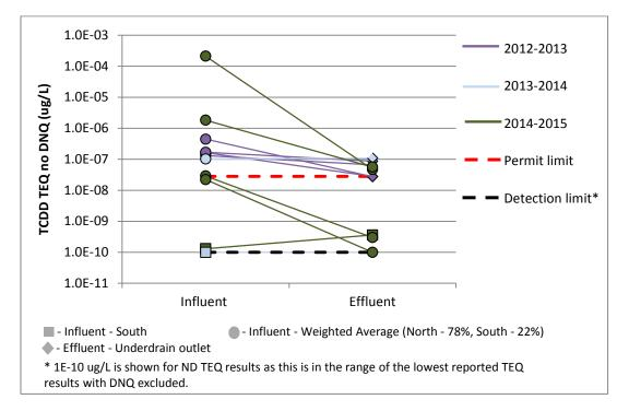
Figure 18. Dioxins at B-1 Media Filter (CM), post curb cuts
