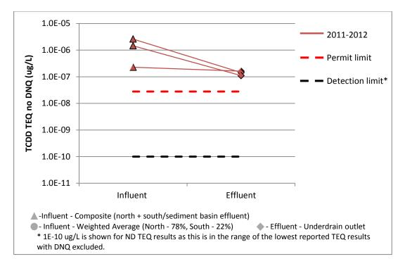
Figure 17. Dioxins at B-1 Media Filter (CM), pre curb cuts
