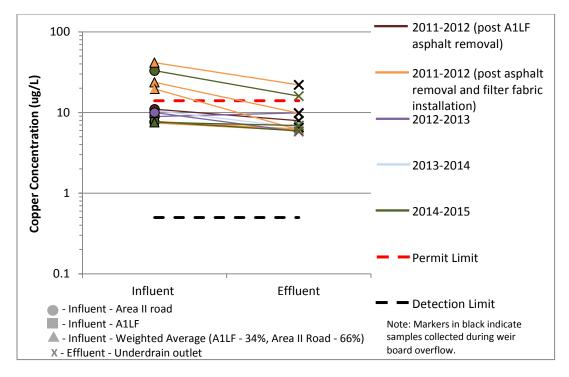
Figure 33. Copper at CM-9, post improvements (removal of A1LF asphalt and addition of CM weir board filter fabric)
