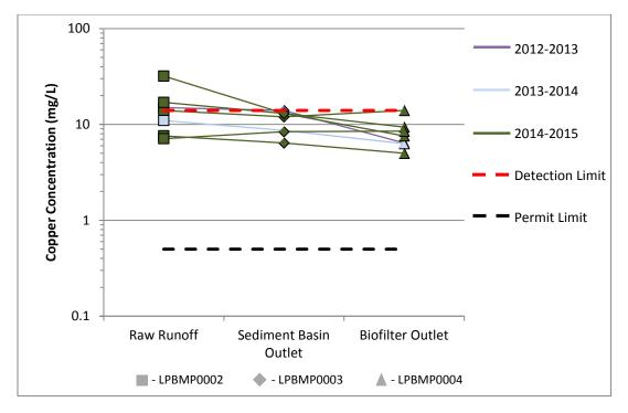
Figure 37. Copper at Lower Lot Biofilter<sup>7</sup>
