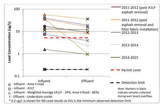
Figure 25. Lead at CM-9, post improvements (removal of A1LF asphalt and addition of CM weir board filter fabric)
