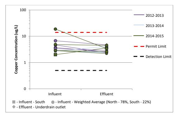
Figure 35. Copper at B-1 Media Filter (CM), post curb cuts
