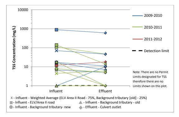
Figure 1. TSS at CM-1, pre filter fabric installation
