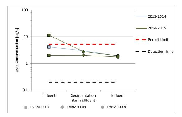
Figure 28. Lead at ELV treatment BMP
