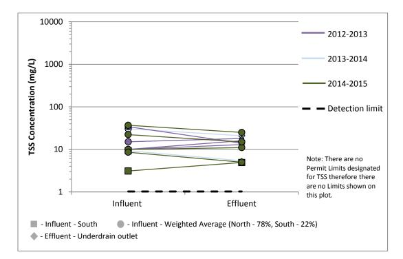
Figure 8. TSS at B-1 Media Filter (CM), post curb cuts
