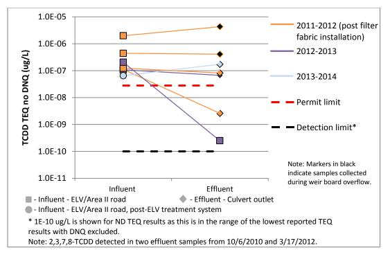
Figure 13. Dioxins at CM-1, post filter fabric installation
