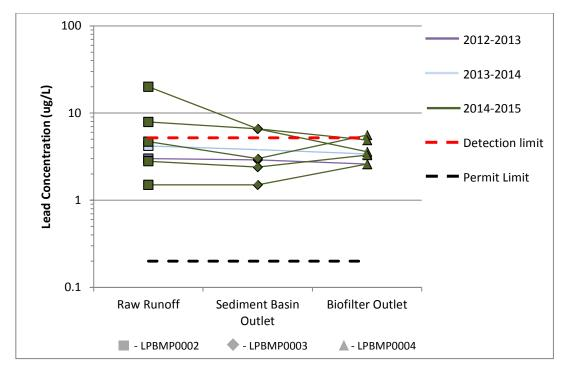
Figure 29. Lead at Lower Lot Biofilter<sup>7</sup>
