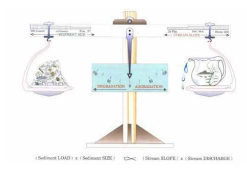
Figure 5 - Schematic of the Lane Relationship After Lane (1955) as cited in Rosgen (1996)
