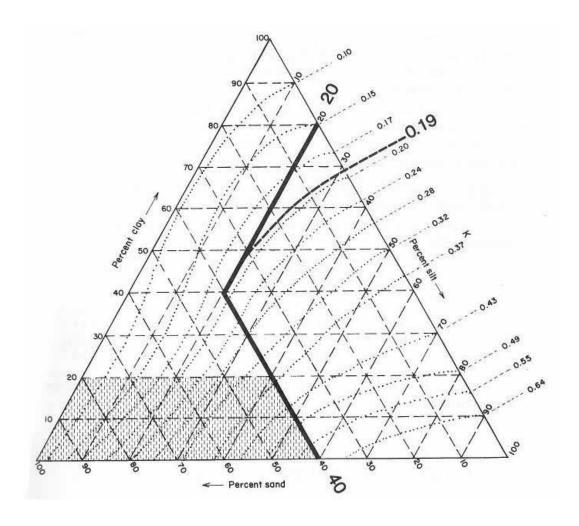
Erickson triangular nomograph used to estimate soil erodibility (K) factor. The figure above is the USDA nomograph used to determine the K factor for a soil, based on its texture (% silt plus very fine sand, % sand, % organic matter, soil structure, and permeability). Nomograph from Erickson 1977 as referenced in Goldman et. al., 1986.
