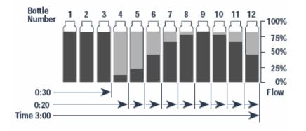
Figure C-7. Sampler schematic for first flush and flow-weighted samples (ISCO)
