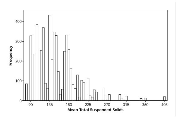
Figure C-4. Histogram of possible TSS concentrations in Flagstaff Street based on collecting three samples per year for two years (the measured median TSS concentration was 170 mg/L)
