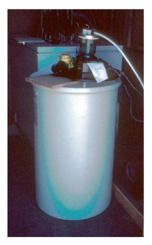
Figure C-5. Automatic sampler with large base for monitoring wide range of flows, with large chest freezer USGS discrete sampler in background, at Bellevue, WA (Pitt 1985)
