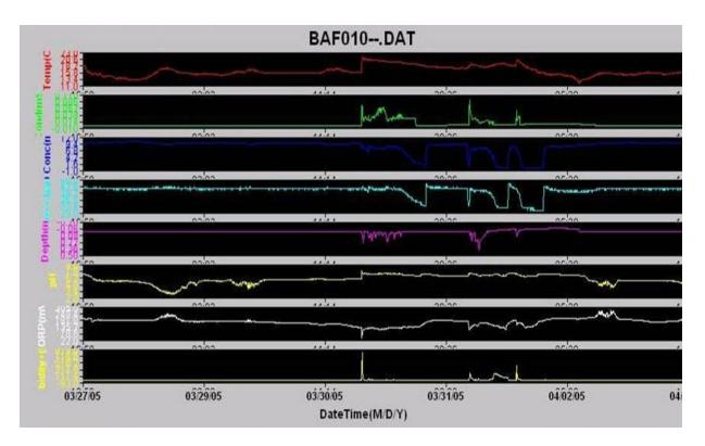
Figure C-8. Screen shot of sonde data analysis screen showing ten days of high-resolution water quality measurements (Pitt and Khambhammettu 2006).
