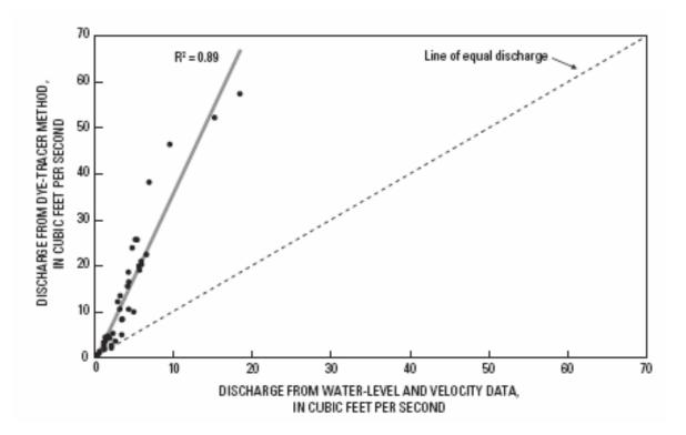
Figure C-1. Relation between actual discharge determined using a rhodamine dye tracer and measured discharge, computed by water-level and velocity data, during free-flow conditions (Selbig and Bannerman 2008).
