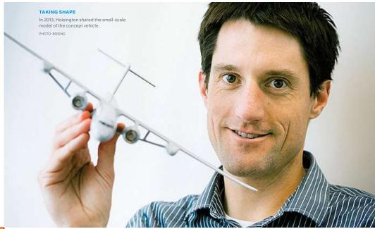
"Adding the truss underneath the wing makes a big triangle. It stabilizes the whole inner part of the wing. The part that's deflecting the most is the part outboard of that. The center is more rigid and the outboard part is more flexible, which mirrors what you see on regular airplanes with cantilevered wings that come out of the fuselage."
