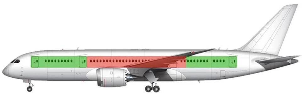
The cut-in area should be forward or aft of the wing.
