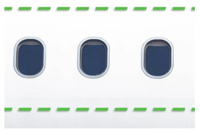
The recommend cut-in area is 12 inches (31 centimeters) above and 12 inches (31 centimeters) below windows.
