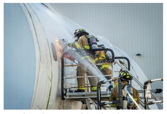
While performing cuts flow water from the crown of the aircraft over the cut area to limit particulates becoming airborne and to control sparking
