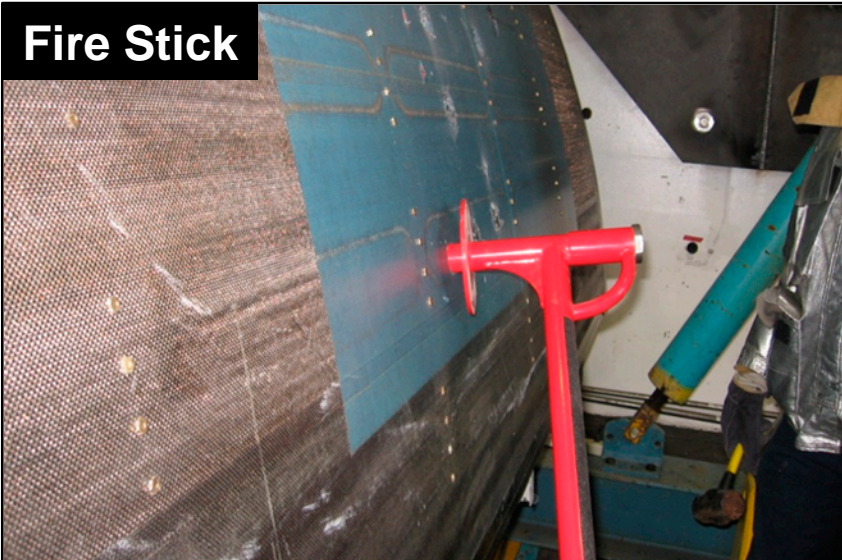
Penetrating nozzle with help of a sledgehammer (interior view)
