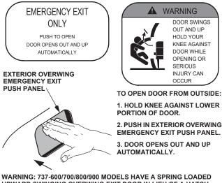
WARNING: 737-600/700/800/900 MODELS HAVE A SPRING LOADED UPWARD SWINGING OVERWING EXIT DOOR IN LIEU OF A HATCH. FOLLOW THE OPENING PROCEDURE INDICATED ABOVE TO AVOID INJURY. 2 FWD AND AFT ENTRY DOOR EXTERNAL HANDLE (LH SIDE)
