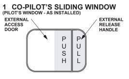
TO OPEN WINDOW FROM OUTSIDE: 1. PUSH IN EXTERNAL ACCESS DOOR. 2. PULL EXTERNAL RELEASE HANDLE. 3. SLIDE WINDOW OPEN.
